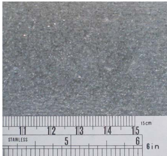
Fig. 5 Spangle-free – Spangles \leq 0.5 mm across
