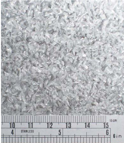
Fig. 4 Small – Spangles up to 5 mm across
