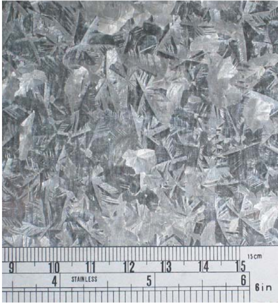
Fig. 2 Large – Spangles \geq 15 mm across
