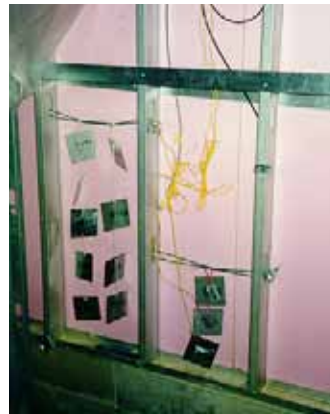
Figure 7 - Wall Cavity Specimens and Sensors in Hamilton, Ontario, Site
