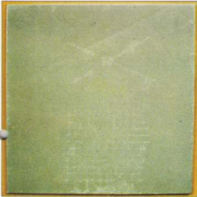
Fig. 1 Acrylic painted galvanized steel — Panel scribed through to steel substrate and salt spray tested to DEF 1053.
