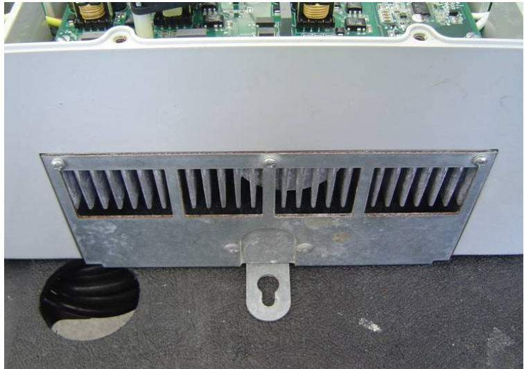
Photo 3 Edge rust on a galvanized part
