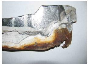
Occasionally, however, galvanized sheet wall cladding, trim items, and stucco flashing comes into contact with soil at lower wall locations. If that happens and the soil gets wet from rain, snow, ice or irrigation, accelerated corrosion can occur as shown in the photo to the left.
