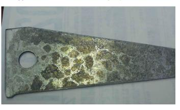
of zinc in the zinc hydroxide, zinc oxide, zinc carbonate sequence that happens over longer periods.
