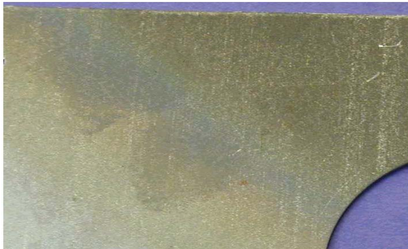
Figure 8 – Storage stain on galvaneal
