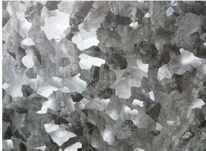
Figure 9 – Severe spangle darkening on galvanized
