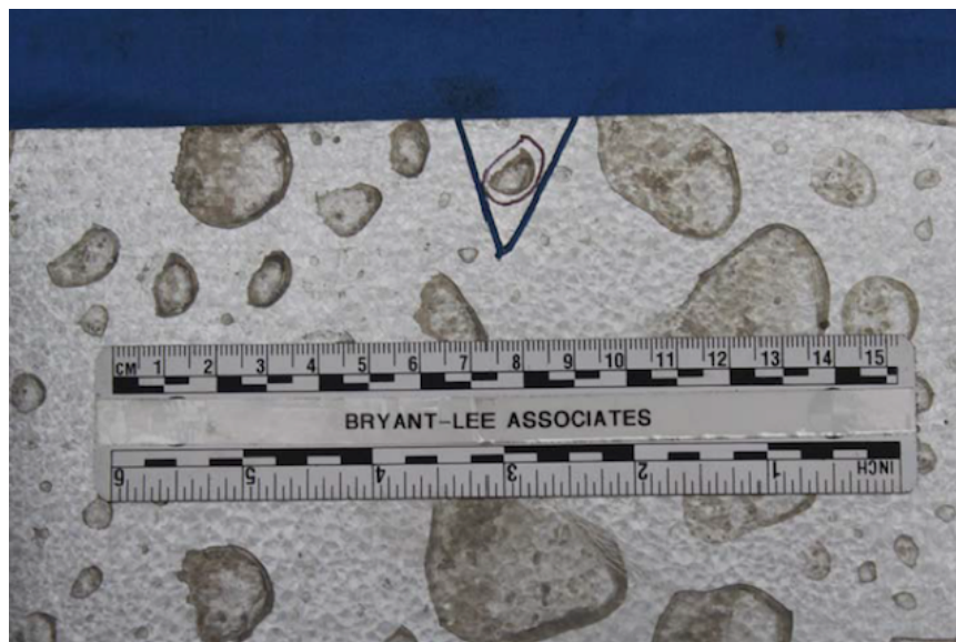
Dried stain on installed AZ standing seam roof panels (September 2013)
