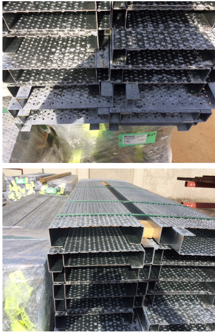
White rust on perforated C channels (February 2015)
