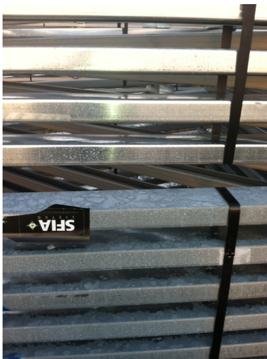
White staining on stacked framing members (December 2013)
