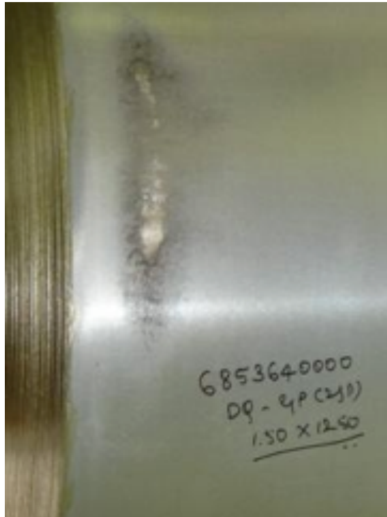
Fretting corrosion (transit abrasion) on a coil of galvanized steel (December 2008)
