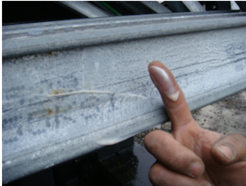
Unknown “foam” on framing after getting wet in the field (January 2008)
