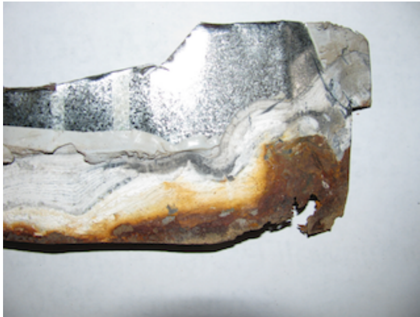
Corrosion on galvanized flashing close to the ground on a stucco wall (April 2010)
