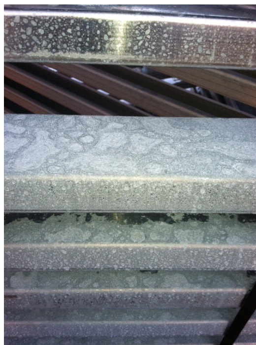
White staining on stacked framing members (December 2013)
