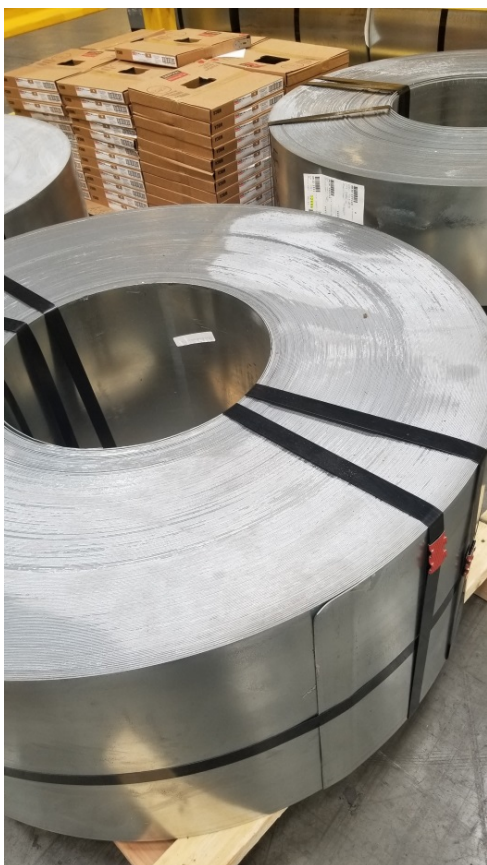
White rust on the edges of slit coils after a 3+ day truck shipment from Stockton, CA to Texas (October 2017)
