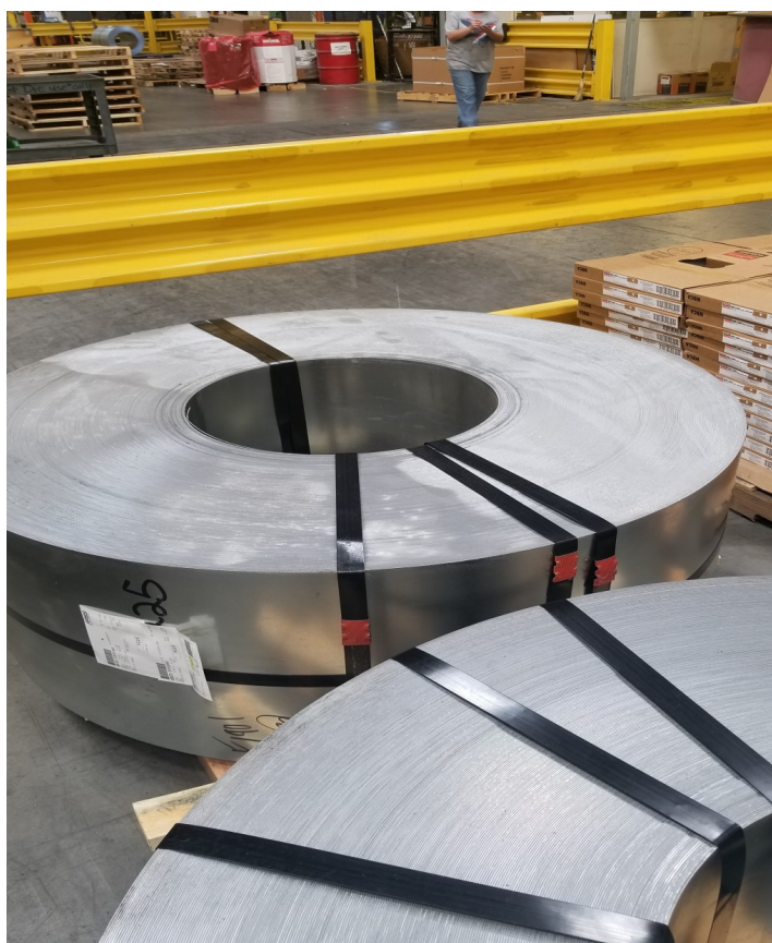
White rust on the edges of slit coils after a 3+ day truck shipment from Stockton, CA to Texas (October 2017)
