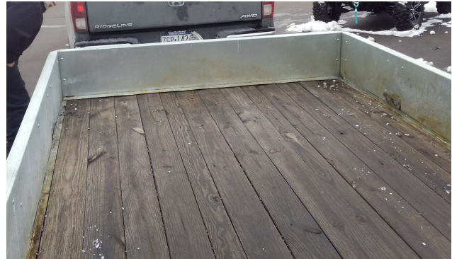
Corrosion on Galvanized Trailer Sidewalls (February 2018)
