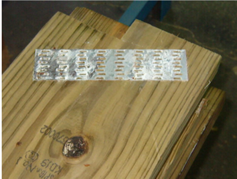
Corrosion of galvanized connector plates used as an anti-split device for ACQ treated planks (October 2005)
