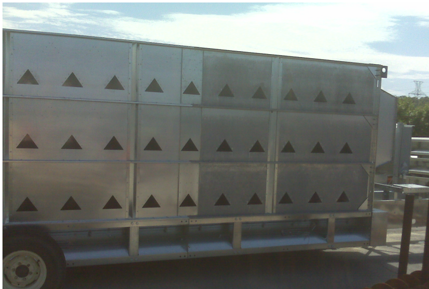
Darkened galvanize (right side) on grain handling equipment (July 2010)
