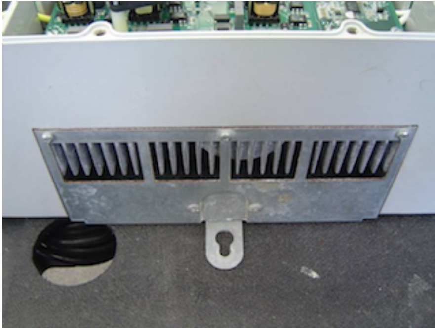
Cosmetic rust on the sheared edges of 0.080" G90 in a greenhouse environment (March 2009)
