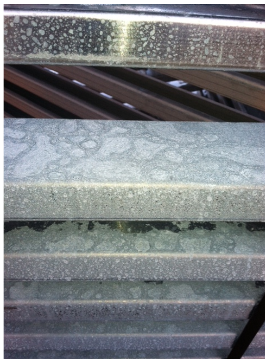
White staining on stacked framing members (December 2013)
