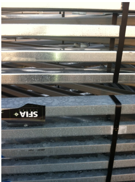
White staining on stacked framing members (December 2013)
