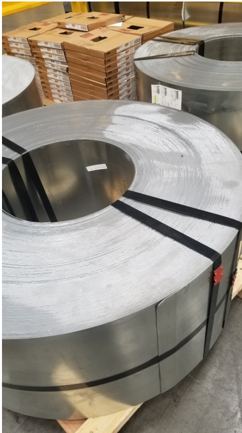
White rust on the edges of slit coils after a 3+ day truck shipment from Stockton, CA to Texas (October 2017)
