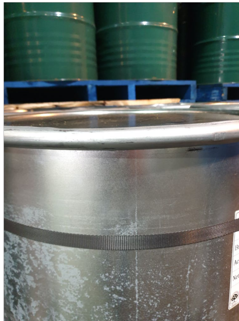
White stains on galvanized drums containing fruit juice (2020)
