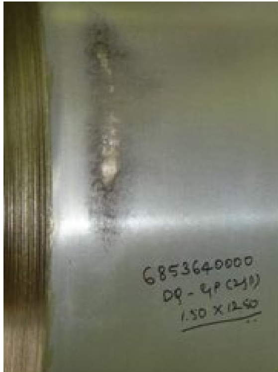
Fretting corrosion (transit abrasion) on a coil of galvanized steel (2010)
