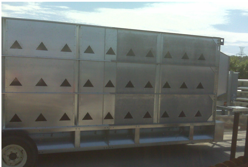
Darkened galvanize (right side) on grain handling equipment (2013)
