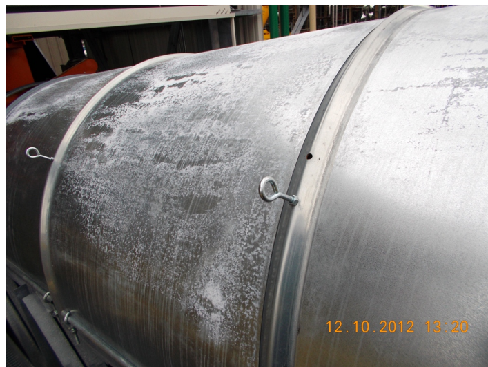
Close-up of storage stain on panels
