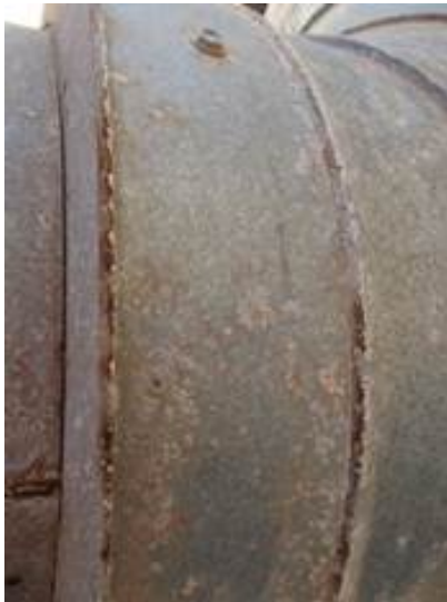
Surface of G90 HVAC located about 1 mile from the coast of Western Australia (October 2015)
