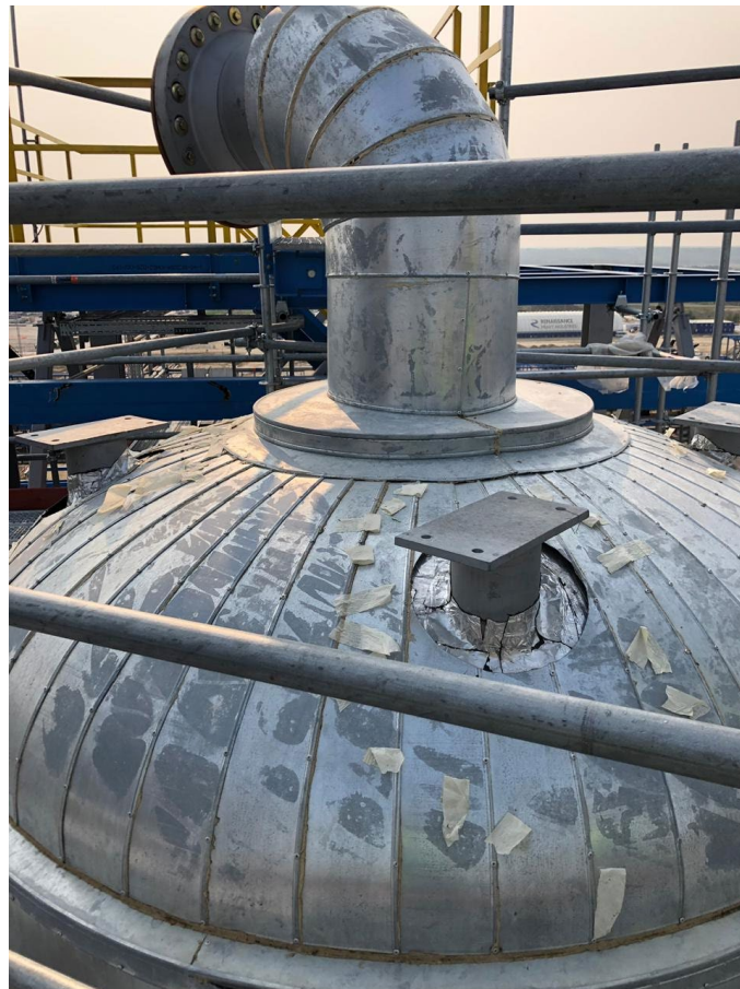
Severe, sudden uneven darkening of galvanized sheet panels on a large refinery installation (2019)
