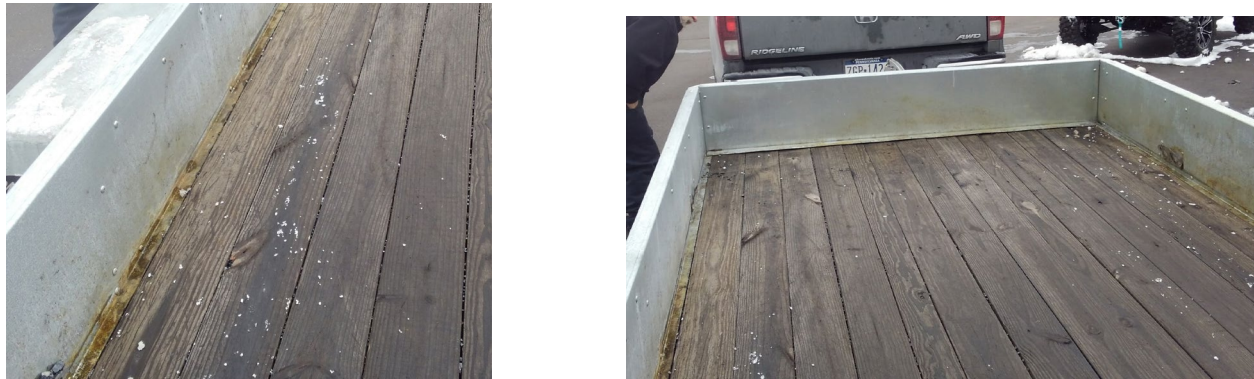
Corrosion on Galvanized Trailer Sidewalls (January 2018)
